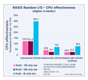
The Graid SupremeRAID solution has much better random I/O CPU effectiveness. This means that more CPU cycles are available for application workload processing for the given storage workload.
