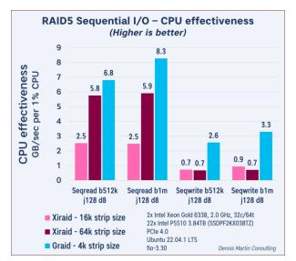
Although the overall sequential throughput results are similar for the two solutions, the Graid SupremeRAID solution has much better sequential I/O CPU effectiveness, especially for sequential writes. As we observed in the random I/O tests, this means that more CPU cycles are available
